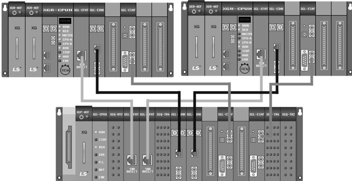
[Fig 6.6.1] Redundant network configuration
