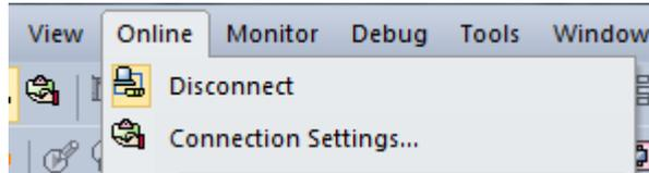
[Fig. 9.2.2] XG5000 remote connection option to select
