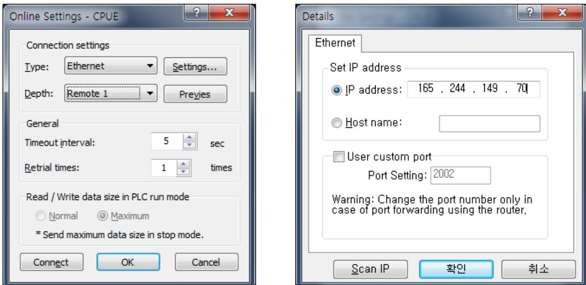
[Fig. 9.2.6] Remote 1 connection directly via Ethernet
