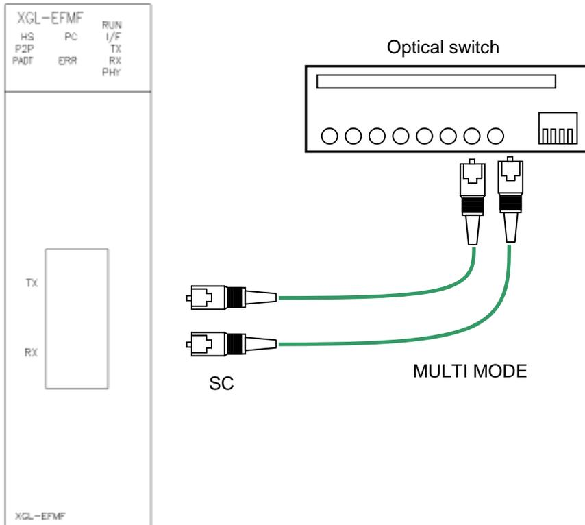
[Fig. 3.2.2] Installation of 100BASE-FX
