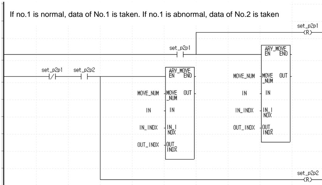
(2) In case XGR and XGK(I) are configured as redundant system with different IP address at the separated network, P2P service connected to Master (standby) is no.1 and P2P service connected to Standby (master) is no.2. If you write ladder about P2P block no.0, you can write the ladder like figure below.
