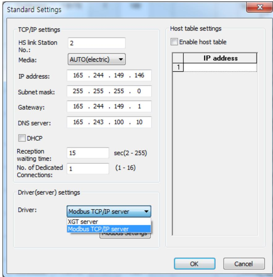
[Fig. 8.3.1] Modbus TCP driver setting
