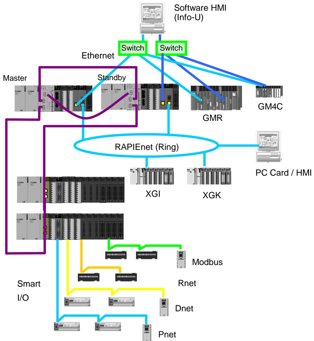
[Figure 4.1.8] XGT redundancy system (Between HMIs, PLCs)
