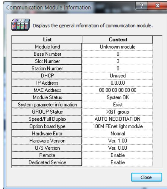
[Fig. 1.4.2] Checking module version through XG5000
