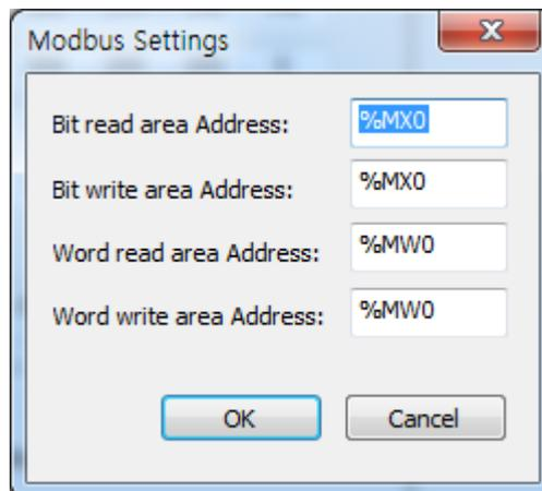
[Fig. 8.3.2] Modbus TCP address
