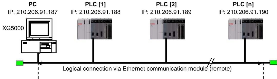
[Fig. 9.2.5] Remote stage 1 connection system through PC
