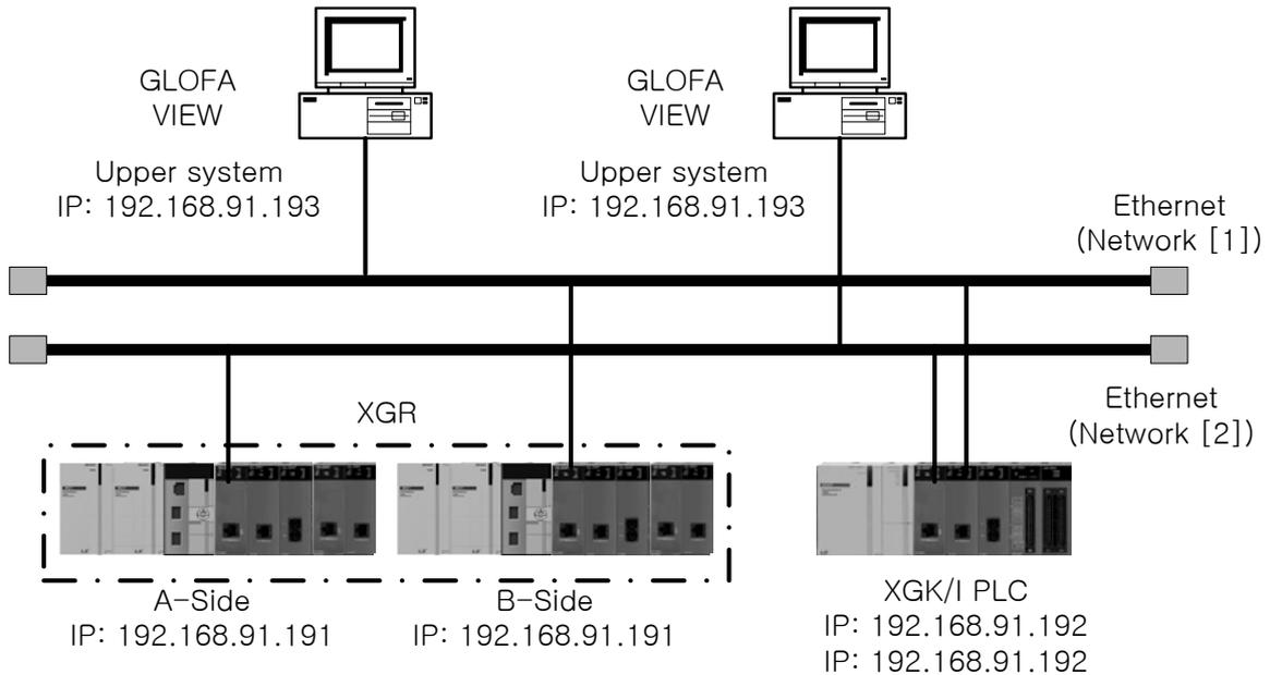
[Figure 4.1.6] XGT Ethernet redundancy system (Redundant Network)
