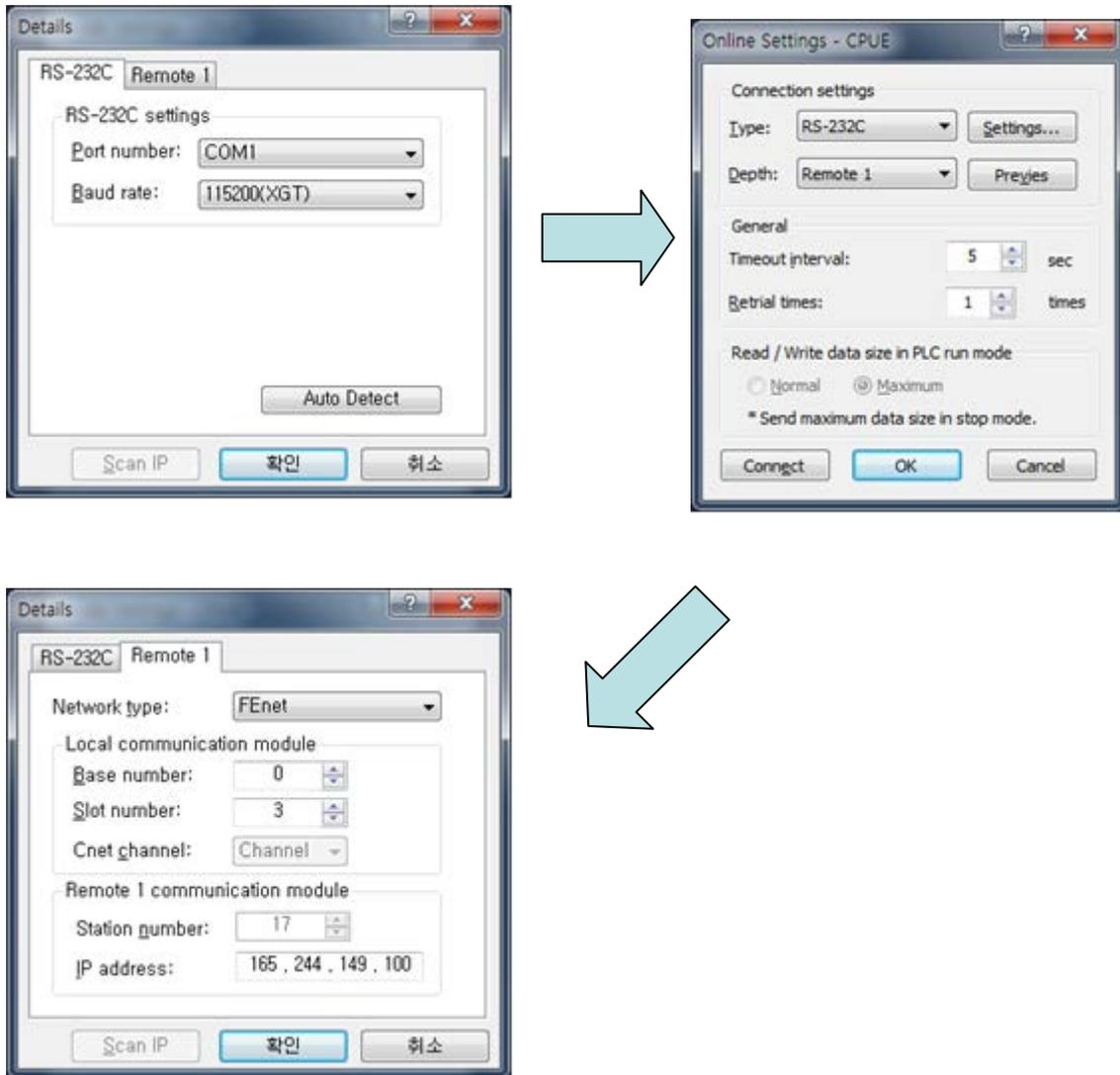
[Fig. 9.2.3] XG5000 remote stage 1 connection
