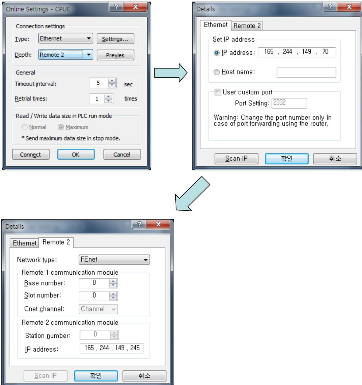
[Fig. 9.2.7] Remote 2 connection directly via Ethernet
