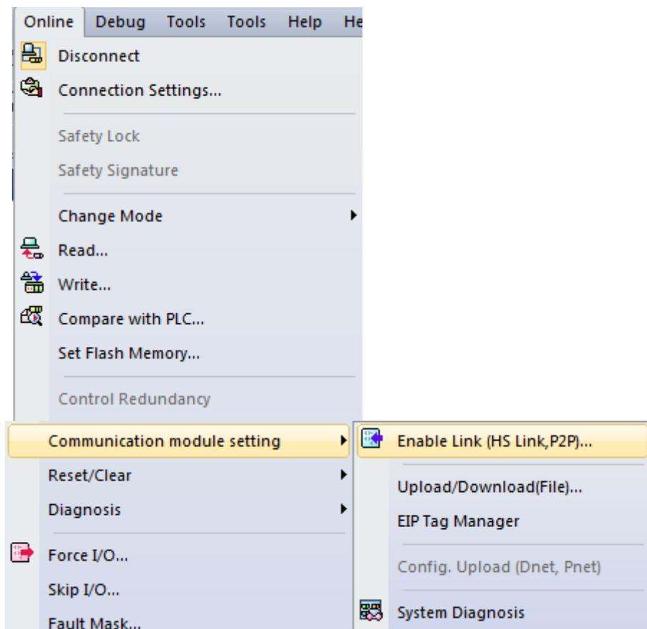
[Fig. 5.5.6] Enable Link setting
