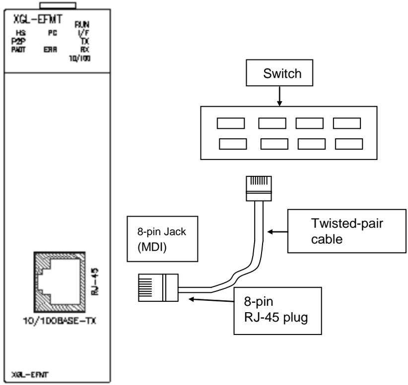
[Fig. 3.2.1] Installation of 10/100BASE-TX
