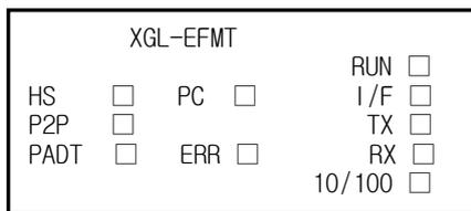
[Fig.10.1.1] LED structure of FEnet I/F module
