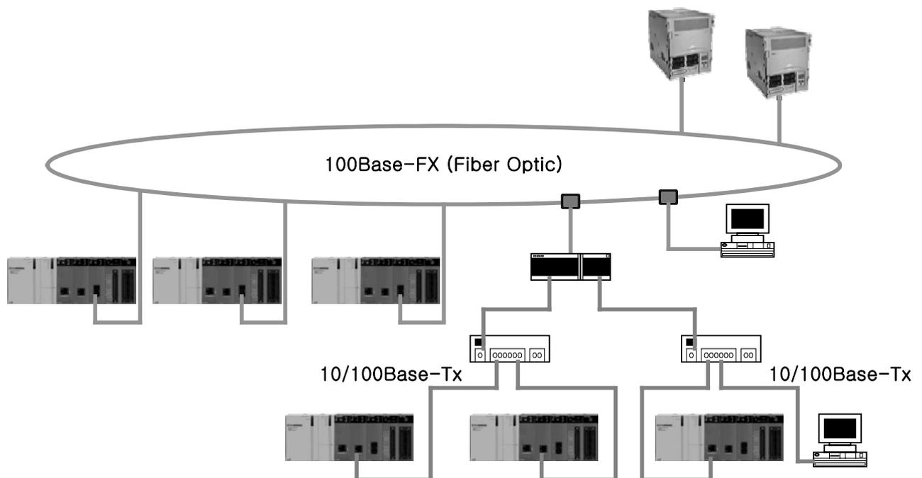
[Fig. 1.2.1] Configuration diagram of FEnet system
