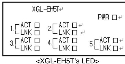
[Fig 10.1.2] LED structure of FEnet I/F module
