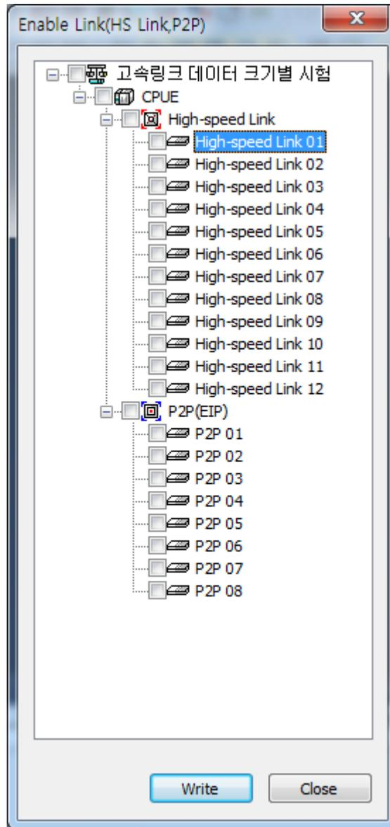
[Fig. 7.4.2] Enable setting of P2P service
