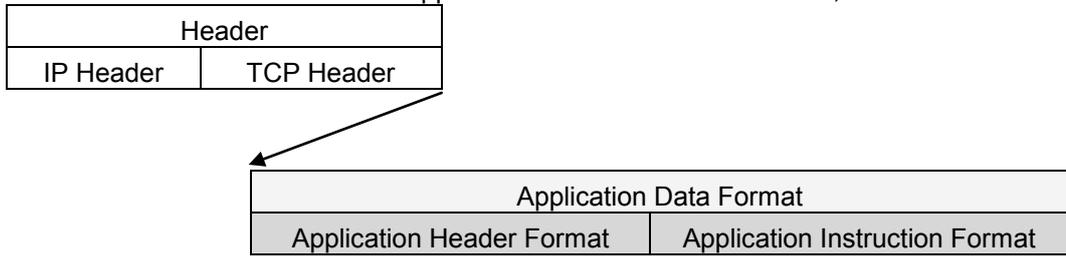
(1) Header Structure (Application Header Format)
