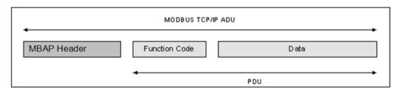
[Figure 5-5] Structure of Modbus ADU
