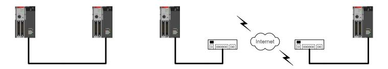
[Figure 4-2] Network configuration using XGB
