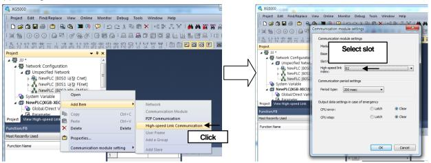
[Fig. 8-2] Setting communication module in HS link parameter
