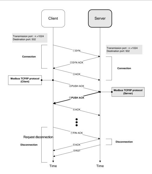
[Figure 6-7] Modbus TCP/IP Server operation flow
