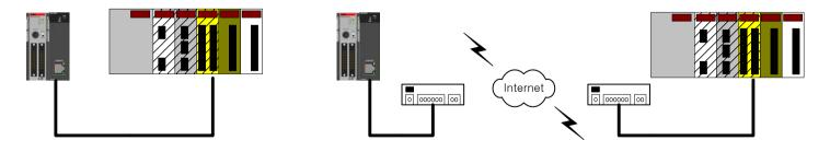
[Figure 4-5] Network configuration using XGB and other LSIS PLC
