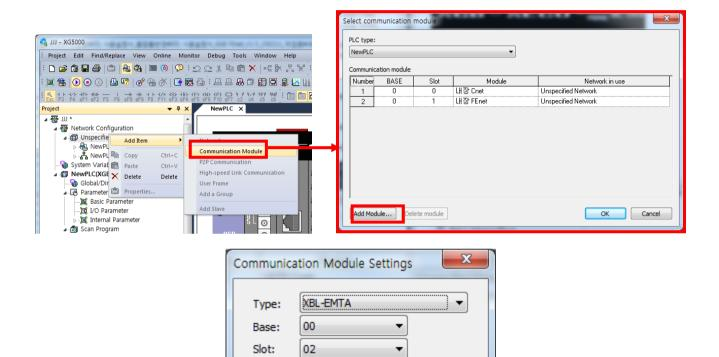
[Figure 6-3] Selecting basic parameter and setting communication module
