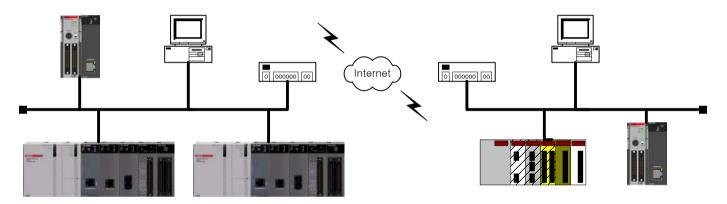
[Figure 4-1] Combination network configuration
