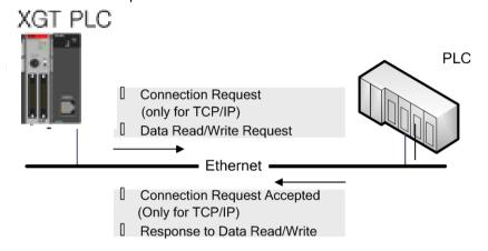
[Figure 7-8] example using P2P channel information
