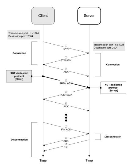
[Figure 7-30] Setting TCP XGT client channel
