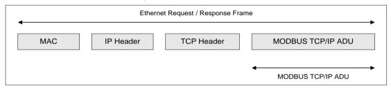
[Figure 5-3] Structure of Modbus TCP/IP frame through Enet
