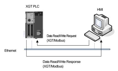
[Figure 7-7] Example of Ethernet (server) driver application
