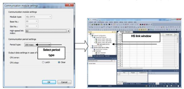
[Fig. 8-3] Finishing HS link communication module setting
