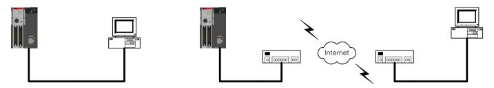
[Figure 4-3] Network configuration using XGB and MMI
