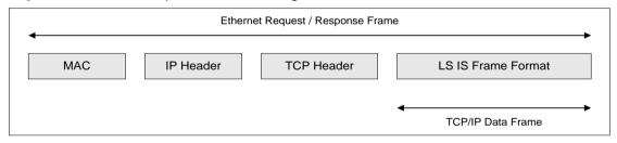
[Figure 5-1] XGT dedicated packet structure through Ethernet
