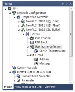
[Figure 7-34] completion of adding the user frame definition group
