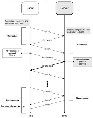
[Figure 6-6] TCP XGT server operation flow
